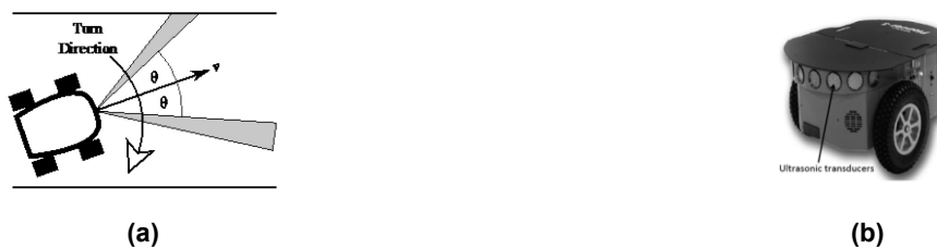
Fig. 5: The robot platform (a) schematic and (b) actual platform using ultrasonic transducers to measure range.
